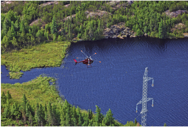
Over 90,000 helicopter hours were logged for tower erection, insulator hanging, transmission line stringing, and transport.
